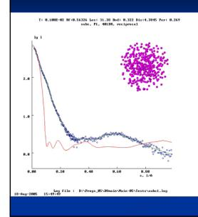
Starting from a random "gas" of 401 dummy residues, fits the data by a locally chaincompatible model
