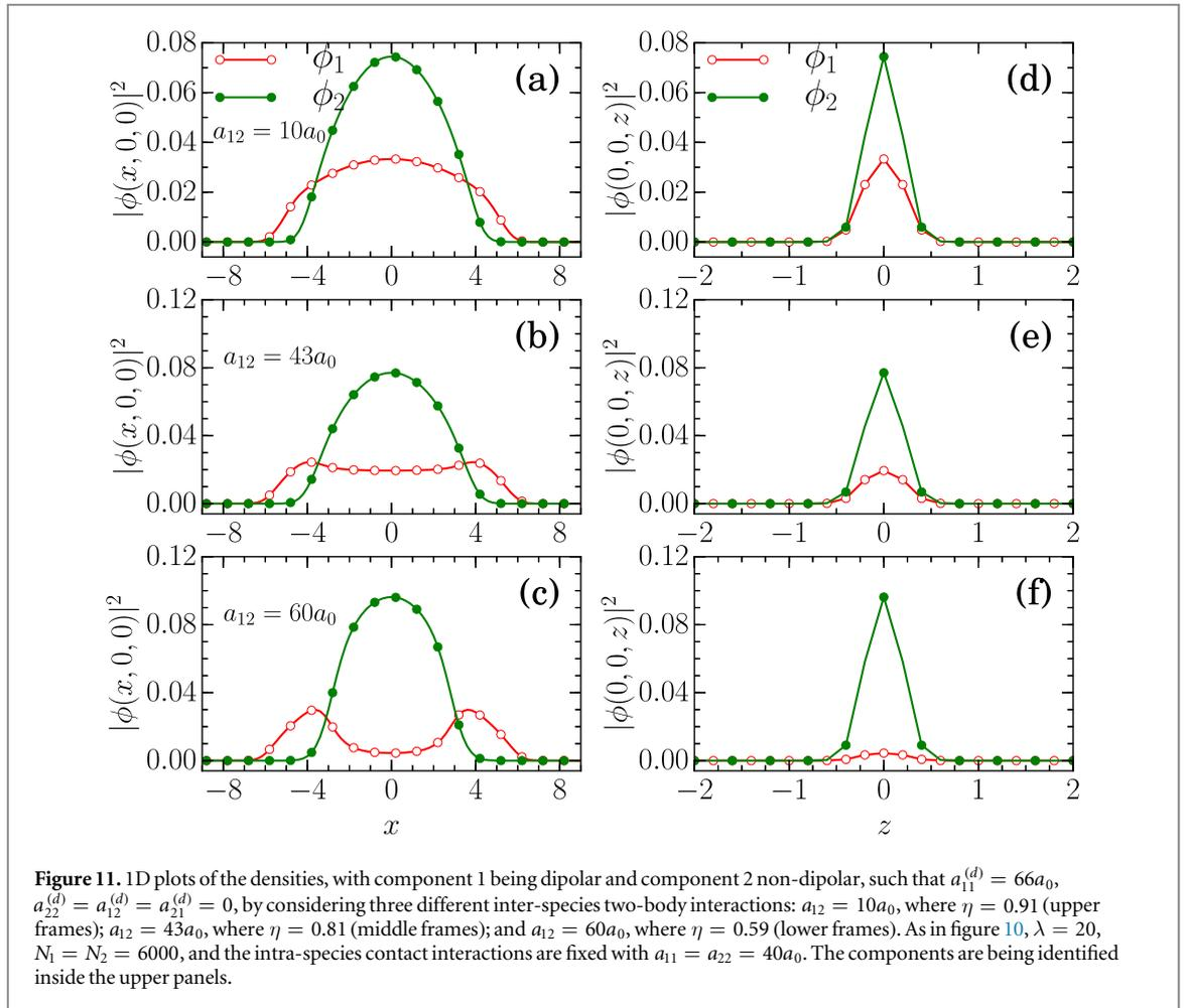
extreme, the system can be considered as almost miscible for  $\eta > 0.7$ . The other intermediate cases can be taken as partially miscible systems.
