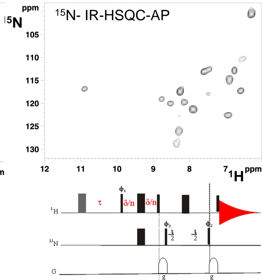
**10 HN peaks, missing in standard  $^{15}\text{N}$  HSQC, can be detected.
